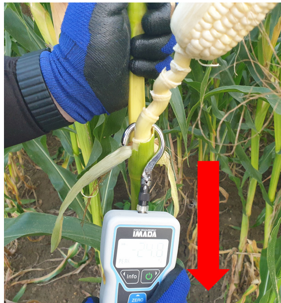
Fig. 3. Detach test of maize sub-stalk and ear.
